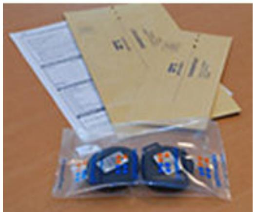
Usually the process begins with the installation of small passive radon monitors. The presence of radon causes invisible damage to the plastic inside the detectors and these changes can be measured and used to calculate the radon level. Analysis and the reporting of individual results are entirely confidential.
